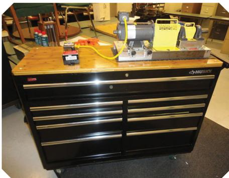
*The results of every change to the simulator is measured providing the positive overall effect on vibration, amps and heat to the bearings. The outcome will prove to participants these techniques work to extend bearing life and improve reliability.*
